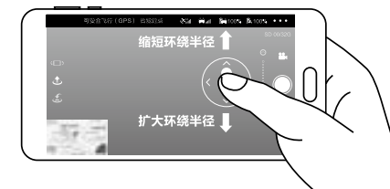
Control the right Joystick to enlarge or shorten the circle radius (Default is the mode 2)
